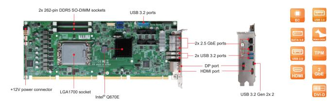
ROBO-8116G2AR is based on Intel® 600 series chipset and workstation processors. Built with flexible PCI express expansions, ROBO-8116G2AR is suitable for Medical, Industrial automation, and Digital Signage application.
